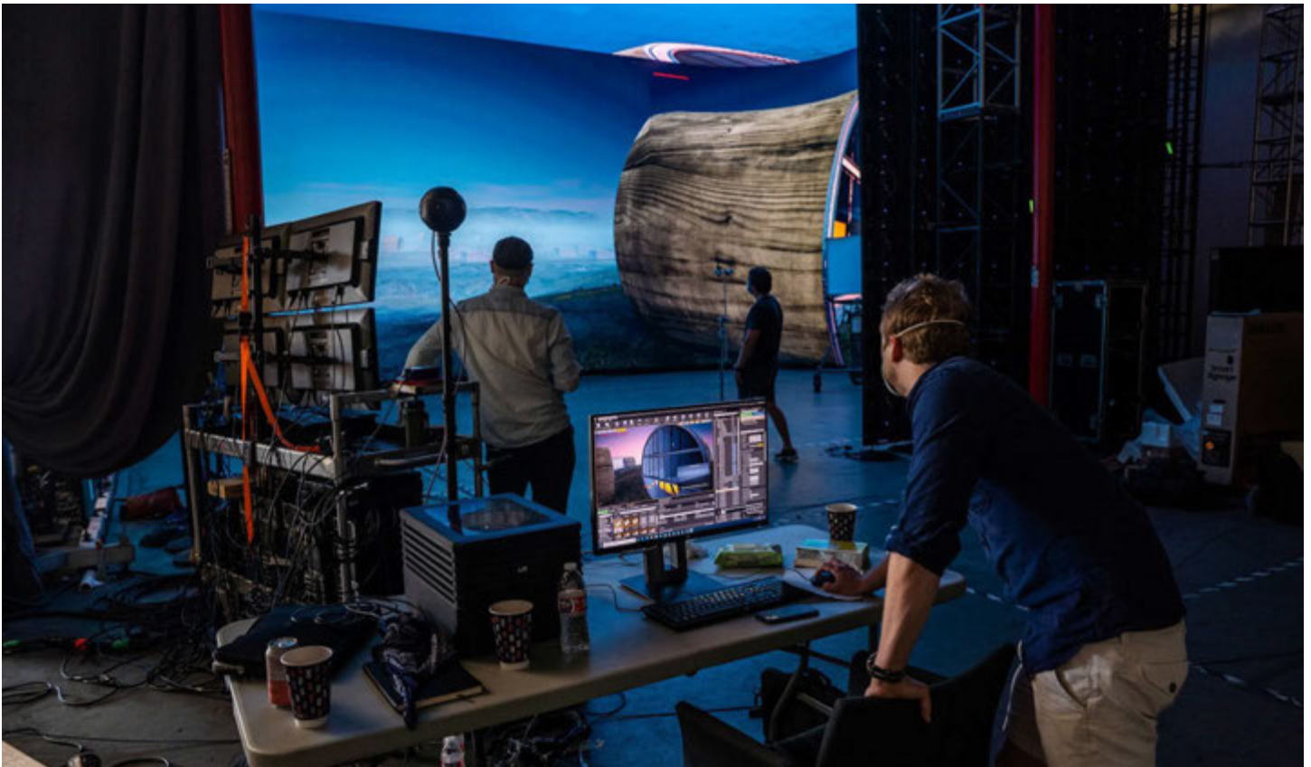
ICVR and Stargate Studios calibrates screen synchronization, content playback frame rate, and camera tracking before the Dining Room Set is built.
