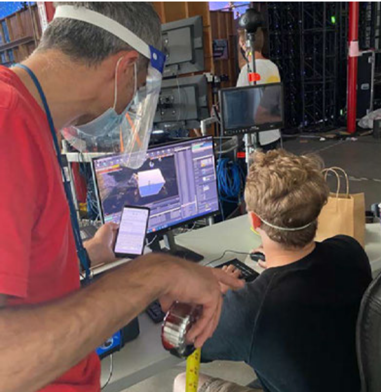
Our VP supervisor worked with ICVR to check scale in our virtual world by measuring physical set piece boxes and making matching CG boxes with the same dimensions.
