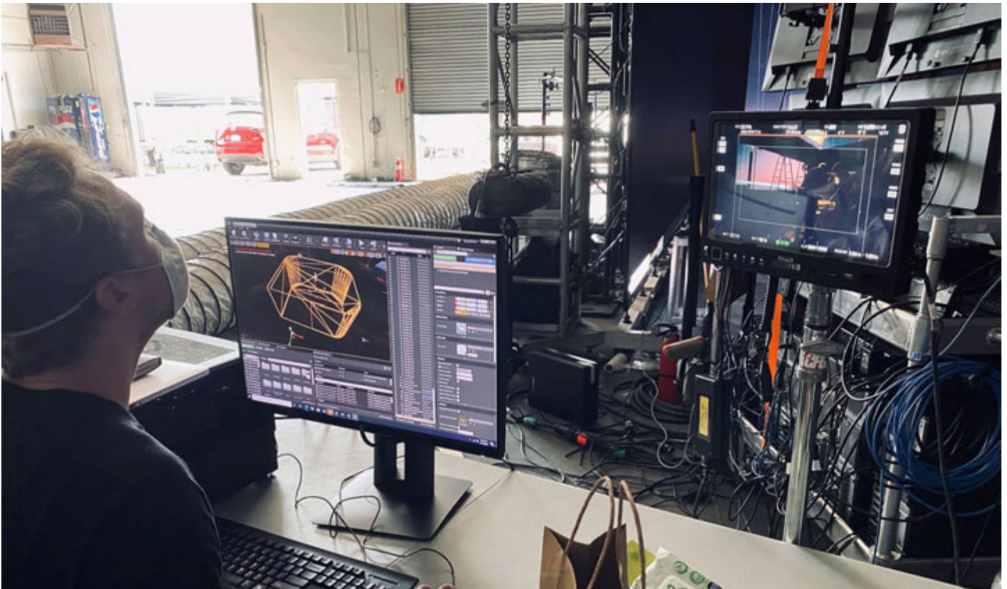
ICVR uses volumetric capture data to align virtual stage with physical stage in Unreal Engine.
